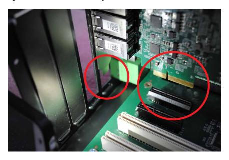
**Step 2.** Make sure edge-finger and PCI Express I/O bracket are inserted smoothly.
