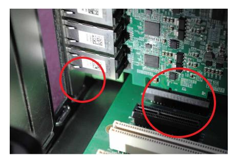
**Step 3.** Make sure PCI Express I/O bracket aligns screw hole.
