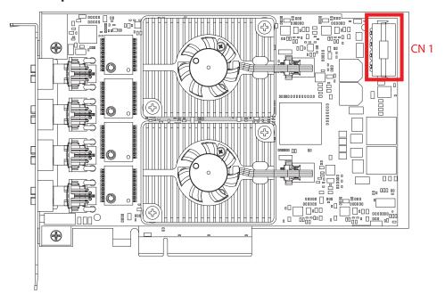
The PE-8004MX is also equipped with one 4-pin power plug (12V, 6A max) for additional power supply. For most cases, the power obtained from PCIe bus is sufficient for the PoE devices, and you do not need to supply extra power to the card. In case the external power is needed, you can use 4-pin ATX power connector (+5V/Red, GND/Black, GND/Black, +12V/Yellow) inside the host computer. Please always confirm the polarity before you plug into the onboard 4-pin power plug.
