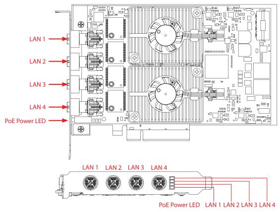
PE-8004MX is equipped with 4 IEEE 802.3at PoE+ ports for transmitting power as much as 25.5W / 48V per port and 1G/10GBASE-T gigabit data signals over standard Ethernet CAT-5/CAT-6 cable.
