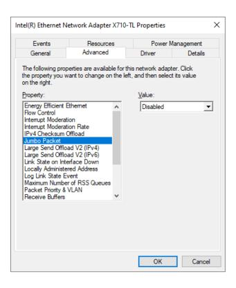
**Step 3.** Select the "Jumbo Packet", settings, and select the expected jumbo frame size and then go "OK" Finish.
