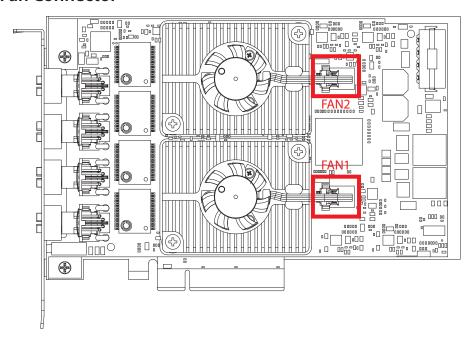
Fan power connector supports for additional thermal requirements. The pin assignments of FAN1/ FAN2 are listed in the following diagram : Pin input :
