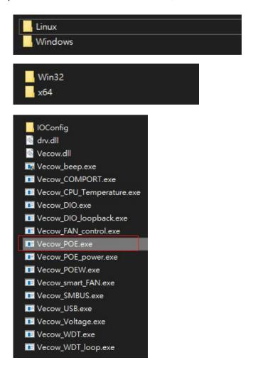
PE-8004MX default is Auto power detect mode, you can use the following software control to switch to manual mode.
